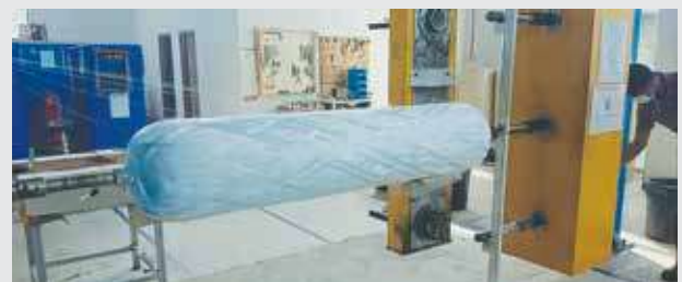
Fabrication of cylinders by filament winding process at STV Permatang Pauh
