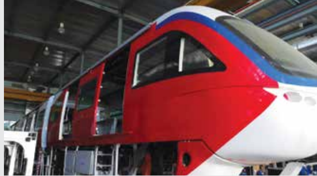
Monorail Assembly Work
