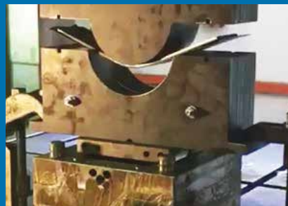
Forming operation of special pipe support
