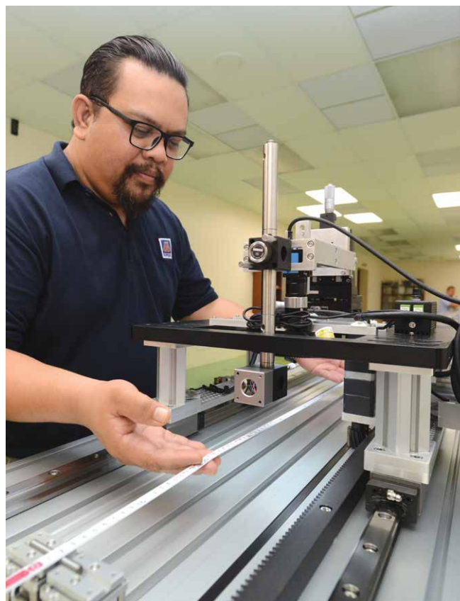
25m Linear Interferometer Bench System at the Dimensional Laboratory
