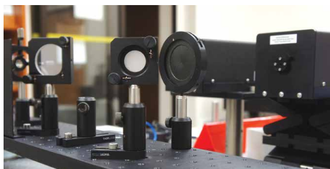
25m Linear Interferometer Bench System at the Dimensional Laboratory
